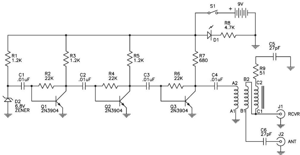
Figure 1: K7QO Noise Bridge Schematic.
