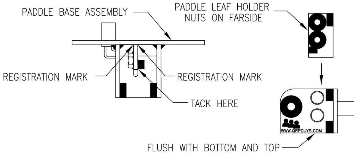
Next, the two **brass** 4-40 nuts need to be permanently soldered to the “inside” of both the contact holders. Use the 4-40 x 3/8”L SS screw, and, a #4 lock washer to hold them in place, and solder the brass nuts to the PCB. *The lock washer insures that the nut will be flush with the PCB when it is heated.* Rub the face of the nut on some scotchbrite or emery paper to clean up the surface contacting the PCB.
