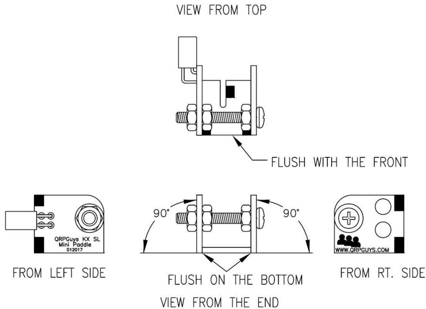
Once all this is aligned and secured, place on a flat surface, and put a "small" tack between each contact holder and the support. *Leave the support screw in place.*
