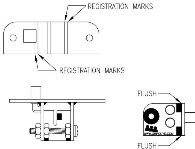
Next, solder the two 2-56 **brass** nuts to the **paddle leaf holder**. Use the two 2-56 stainless steel screws to secure the brass nuts on the side of the paddle leaf holder marked “**nuts**”, and solder the brass nuts to the PCB. *The lock washer insures that the nut will be flush with the PCB when it is heated.* It is helpful to rub the face of the nut on some scotchbrite or emery paper to clean up the surface contacting the PCB.
