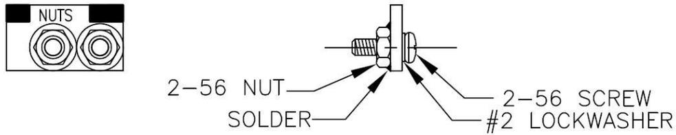
Next, position the paddle leaf holder with the nuts into the contact holder/support assembly as shown below, flush with the top, bottom and paddle base assembly. And yes, it is supposed to be snug in the support slot , to hold it in position while you solder. Tack one spot in place and check for alignment with the registration marks, re-heat and adjust if necessary. Tack all the remaining pads, then finish soldering the pads.
