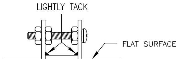
Next, position the **contact holder/support assembly** on the **paddle base** with the registration marks, and lightly tack a couple of points on the ends. The female 2x2 header should be centered in the cutout. If all looks good, tack both sides of the holders, and alternate back and forth between the two sides adding a little more solder. Finish soldering all the pads, and then remove the support screw.
