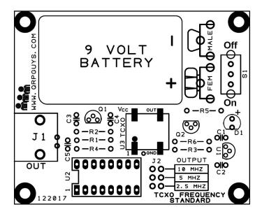
[ ] Install U3, 20MHz TCXO, put a small drop of solder on pad #1 of the pcb, center the chip on the outline and solder that pad. Solder the remaining 3 pads.
