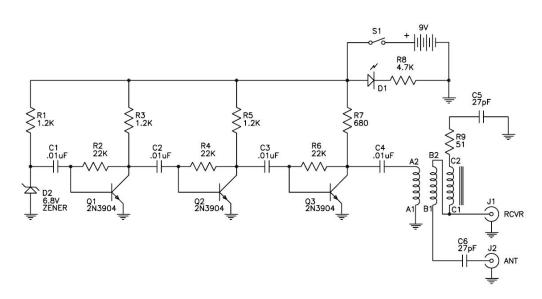
Figure 1: K7QO Noise Bridge Schematic.
