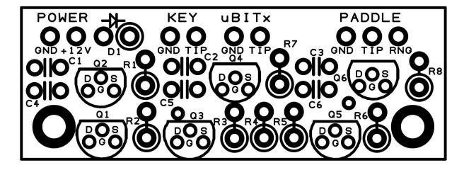
All the components mount of the top side of the board. There are two #2 clearance holes for mounting.
