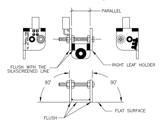
Mate the previous assembly to the **paddle base** as shown in the figure below. Align registration silk screened lines and flush on the top and bottom. Tack one small joint and check for alignment. When you are satisfied with the alignment, lightly tack all the other points. Finish soldering all the pads, including the joints between the leaf holders and the contact holder. You may now remove the 2-56 screw and nuts.
