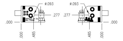
ADD A Ø3/32" HOLE ON EACH SIDE AS SHOWN
