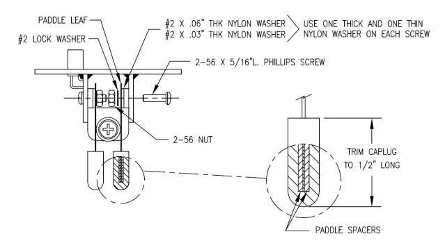
Cut the vinyl caplug lever cover 1/2" long from the closed end with scissors or a razor knife. Cut the piece of 1/2" wide plastic into two 7/16" long pieces. Sandwich the paddle lever between the plastic spacers and slide the caplug over the end of the paddle leaf.
