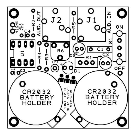
We have designed the board to be used outside, on battery power, or mounted inside your transceiver running from power obtained from your transceiver. We suggest building it as an outside device, and it is easily transformed if you decide to mount it internally.
