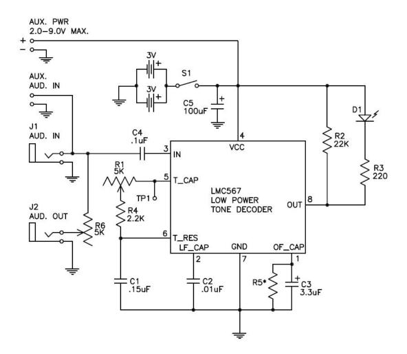
We included a position R5 for experimenters that want to try different sensitivities. According to the LMC567 specification sheet, "Pin 1 also provides a means for shifting the input threshold higher or lower by connecting an external resistor to supply or ground. However, reducing the threshold using this technique increases sensitivity to pin 1 carrier ripple and also results in more part to part threshold variation." The full spec sheet can be downloaded from our Misc. Files tab.
