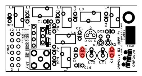
[ ] Install C7, 680pF, mono capacitor, marked 681
