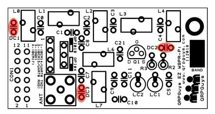
[ ] Install C0,4, 390pF mono capacitor, marked 391
