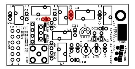
[ ] Install C2, 470pF mono capacitor, marked 471
