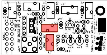
[ ] Wind L1 and L3 using 6" for each, of the supplied magnet wire and a FT37-61 (black) toroid with 7 turns as Shown below. Tin the leads before installing.
