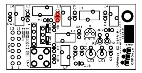
[ ] Install C5,11, .01 mono capacitor, marked 103
