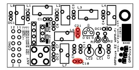
Use caution identifying the inductors and resistors. They are difficult to remove if installed in the wrong location. Bend as shown and the end of the component mounts flush with the board at the silkscreened circle.
