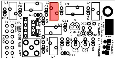
[ ] Wind L0 and L4 using 7" for each, of the supplied magnet wire and a T37-6 (yellow) toroid with 10 turns as shown below. Tin the leads before installing.
