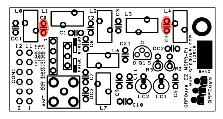
[ ] Install C1,3, 39pF, mono capacitor marked 39
