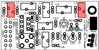
[ ] Wind L6 and L7 using 9" for each, of the supplied magnet wire and a T37-6 (yellow) toroid with 14 turns as shown below. Tin the leads before installing.
