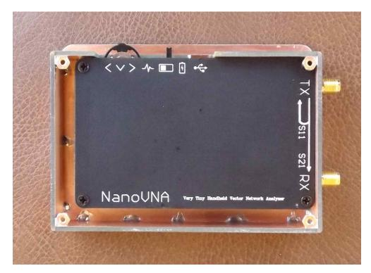
From the pictures above and below you can see there is about a 1/4" extra space on two sides to allow room to get the device into the new chassis. Also, you can see how the back panel and the same size cover will protect the rocker switch and slide switch. There is also more room in the overall thickness to replace the LiPo battery to one of more capacity.
