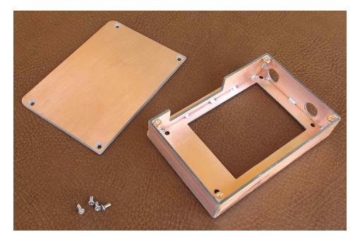
The original front plate shipped with the NanoVNA is not used. This allowed me to use the four corner screws to secure it to the new chassis. The original is removed and not used in the new setup. You may use it however if you want to transfer the hole and window locations to the new front plate.
