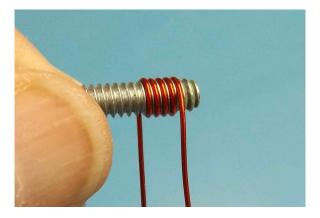
Trim both primary and secondary to 9/16" length and tin 1/8" of the lead ends as shown below.
