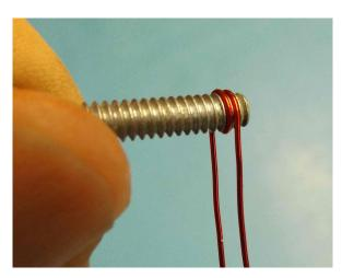
[ ] Wind the Secondary, (4 1/2 turns) on the supplied screw into the grooves of the screw thread as shown below, with the 22awg magnet wire.
