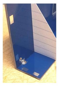
Check it for squareness right beside where you did the light tack. If it is not square, simply reheat the pad and reposition until it is square. Change wire diameter if necessary, re-check with your inspection tool, and repeat until both places are square. You must re-heat the joint every time you want to make an adjustment. Use the same technique for the center joint. Leave the three joints lightly tacked. Do not go back and finish solder, we'll do that later. Save the gage.
