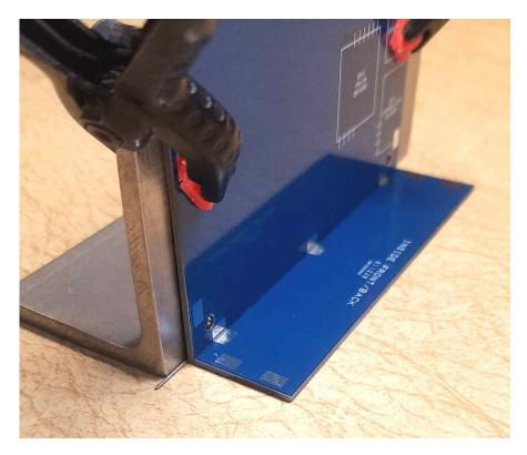
Here the bottom is against angle iron, and the front pcb is flat on the table.
