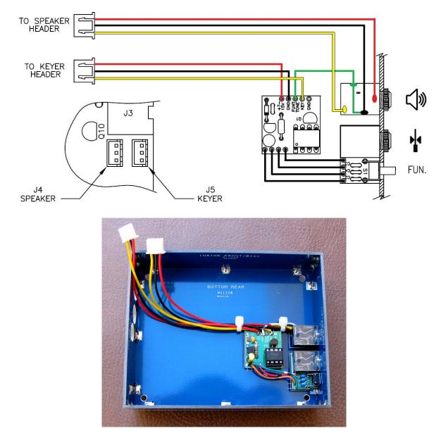
Wiring note: The speaker jack is shown facing up for connection clarity. Install the jack with the pins down.
