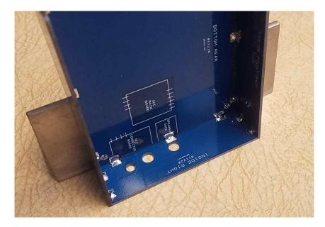
[] Turn the partial assembly over and apply the same assembly technique to the left side pcb.
