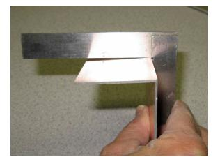
We need to allow for this change. You will do it by pre-positioning the clamped angle to slightly greater than the desired 90°. By clamping the bottom pcb against the angle iron, with an approximate 1/32" diameter piece of solder or wire between the outside of the pcb and angle iron, it tilts back the pcb to greater than the needed 90° angle. When this joint is soldered it will draw back to a 90° corner. See the sketch below.
