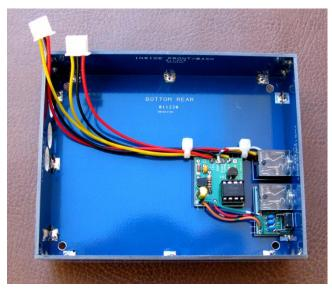
Use the two 4" cable ties to bundle the wires close to the pcb. This reduces the strain on any individual wire.
