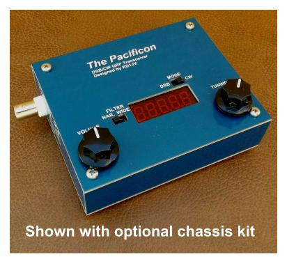
Featuring: Wide tuning range digital VFO with 5 digit LED readout.
