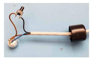
5. Slide the assembly into the tube, and let the switch post come thru the squared hole and epoxy in place. Let the epoxy harden. Be careful not to get any epoxy surrounding the switch post.
