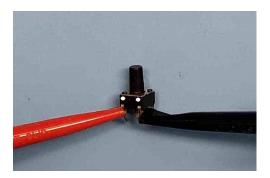
4. Wire according to the schematic, and double check the wiring before you epoxy the switch in place. The electret element is polarity sensitive. Use the manufacturers drawing for determining the polarity. If unknown, the pin that has continuity with the outer case is usually (-).
