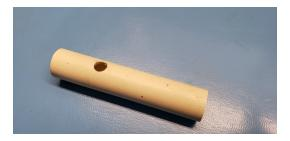
2. Square up the hole with an Xacto knife so the N.O. switch just can pass thru the hole. It will be epoxied in place eventually.
