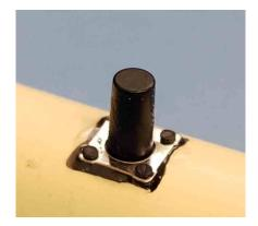
6. Push the microphone into the end of the tube so the face of the microphone is about 3/16" inside the tube and epoxy (X-X) in place. Let the epoxy harden.
