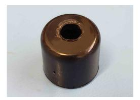
8. Install the cap with the 1/4" hole on the microphone end. Pass the microphone cable thru the inside of the other cap. Tighten the 1/8" Tyrap on the inside of the cap to act as a strain relief for the cord and install the other vinyl cap.
