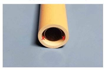
7. With your soldering iron, make a hole in the center of one vinyl cap about 1/4" in diameter for the microphone end. In the other cap make a hole of a diameter that will just allow the three conductor cable to just pass through.
