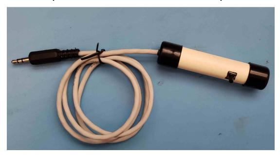
You can easily fabricate an electret PTT microphone with common household tools.
