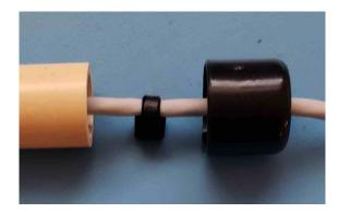
9. Wire the 3.5mm stereo plug sleeve, ring, and tip, according to your circuit requirements.
