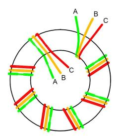
Bend the wires down and pre-tin the wire in preparation to soldering them to the board. Solder the toroid flush with the top of the board. Shown below is how it should look when soldered into the board.
