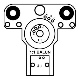
First to install is T1 that must be wound as shown below.
