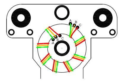
[ ] Retain T1 with the two nylon tie wraps as shown below.
