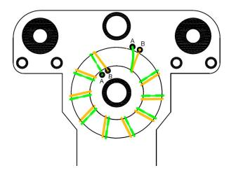
[ ] Retain T1 with the two nylon tie wraps as shown below.
