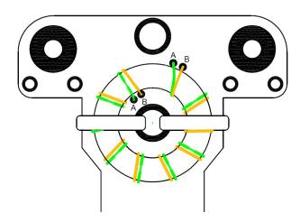
[ ] Install the hardware posts for the antenna and counterpoise wires on the top of the board, as shown in the figure below. The post screw should be flush with the outside of the securing nut on the bottom side.
