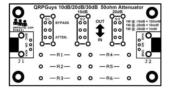
All the components mount of the top side of the board, except the rubber feet, unless you are planning to mount the device in a chassis. In that case, mount the switches on the top side, and the connectors and resistors on the back side.
