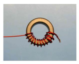
[ ] The next turn will cross down through the center of the core 180° and cross to the other side of the toroid as shown. Because it goes thru the center of the core, it counts as the **13th turn** of the secondary.
