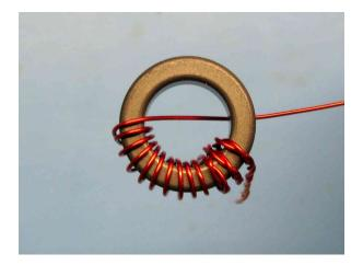
[ ] Now pass the wire **down** through the center of the core and wind in a counterclockwise Direction for another 11 turns. This will result in total of a **24 turn** secondary, as shown below.
