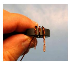
[ ] Continue winding the secondary with the loose end of the wire passing **down** through the center of the core, winding (clockwise). The picture below shows first 12 turns of what will be a total of 24 turns for the secondary
