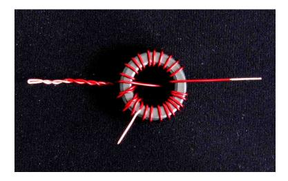
The transformer is now pre-soldered and pre positioned as shown below, with all the connections soldered, except the center BNC pin.
