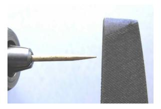
[ ] On the other end, if the rod does not fit into the terminal, file down the brass rod to accept the #6 ring terminal, and solder it in place. The brass rod must be clean to solder.
