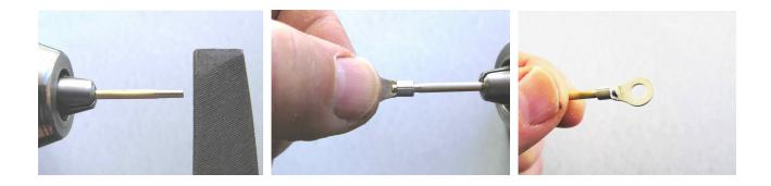
[ ] Use the 6-32 hardware and mount the probe tip to the PCB as shown in the figure below.
