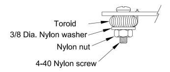
[] Solder L2 where indicated on the PCB, and centered on the screw hole. You will notice the tap hole is indicated, and is slightly larger in diameter to accept the double twisted wire. Install the toroid flush with the backside of the board. Do not elevate it off the board. Secure it the nylon hardware the same as shown above.
