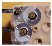
[] Install the polyvaricon capacitor on the "**BACK**" side of the board by carefully bending the three leads towards the shaft end of the capacitor. Feed the three leads through the board and secure it with the two short metric Phillips screws from the top. Solder and clip the three leads flush.
