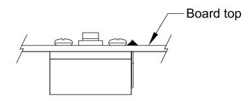
[] Install the slide switch on the "FRONT" side of the board, soldering all four corners and electrical pins.
