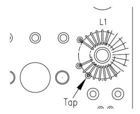
[] Secure L1 to the bottom side of the board using one of the 4-40 nylon screws, nylon washer, and nylon nut, as shown below. Tighten enough to secure and protect the toroid, but do not over tighten.
