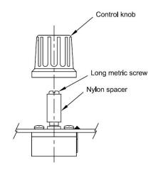
This completes the electrical and mechanical assembly.
