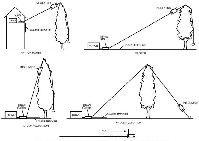
ALWAYS CUT YOUR ACTICE ELEMENT 1 OR 2 FT, LONGER AND WRAP IT BACK UPON ITSELF. THIS LEAVES SOME WIRE FOR ADJUSTMENT. IT STOPS RADIATING AT THE POINT OF THE BEND AT THE INSULATOR. THE INSULATOR CAN BE A SIMPLE 2" LONG PIECE OF PLASTIC TUBING WITH A COUPLE OF HOLES IN IT.
