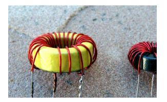
[] Solder L1 where indicated on the PCB, and centered on the screw hole. You will notice the tap hole is indicated, and is slightly larger in diameter to accept the double twisted wire. Install the toroid flush with the backside of the board. Do not elevate it off the board. We will be securing it with a nylon screw, nylon washer and nut.
