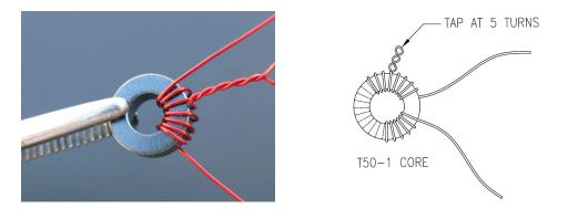
[] Next, bend the leads as shown below, trim to 1/4" long, and tin the leads prior to soldering them to the backside of the board. The magnet wire supplied Is Thermaleze® brand and will tin easily with a soldering iron. Always tin the leads before trying to solder them in place and you will greatly eliminate any continuity problems.
