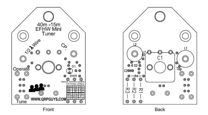
[] Install D1, the clear lens LED on the **"FRONT**" side of the board. The polarity must be correct. The short lead is "negative" and goes towards the top of the board. There is also a very small flat indicating the negative side of the led, and an outline indicating the flat on the board. Seat the LED flush with the surface of the board.
