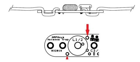
The user supplies the wire for the elements. We recommend stranded #22-24 AWG.
