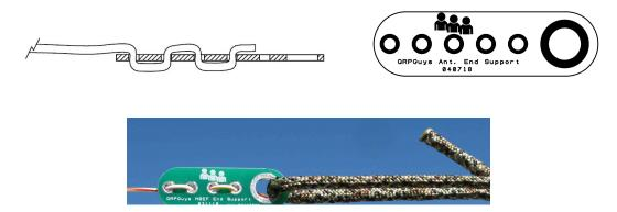
When you are satisfied with the performance, cut a 1.75" long piece of the Ø1/2" heat shrink tubing, remove the End Support, slide the heat shrink onto the end of the wire, center it on the trap, and shrink it to the assembly, as shown below. It will not be waterproof, but it is designed to protect the trap from mechanical damage in the field. Replace the end support.
