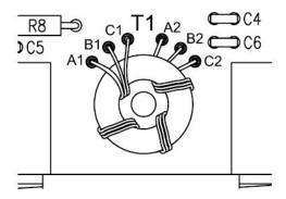
[ ] Secure T1 to the board using the 4-40 nylon screw, nylon washer, and nylon nut, as shown below. Tighten enough to secure and protect the toroid, but do not over tighten.
