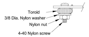
[ ] Solder L2 where indicated on the PCB, and centered on the screw hole. You will notice the tap hole is indicated, and is slightly larger in diameter to accept the double twisted wire. Install the toroid flush with the backside of the board. Do not elevate it off the board. Secure it the nylon hardware the same as shown above.
