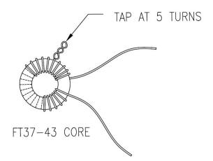
[ ] Next, bend the leads as shown below, trim to 1/4" long, and tin the leads prior to soldering them to the backside of the board. The magnet wire supplied Is Thermaleze® brand and will tin easily with a soldering iron. Always tin the leads before trying to solder them in place and you will greatly eliminate any continuity problems.
