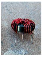
[ ] Solder L1 where indicated on the PCB, and centered on the screw hole. You will notice the tap hole is indicated, and is slightly larger in diameter to accept the double twisted wire. Install the toroid flush with the backside of the board. Do not elevate it off the board. We will be securing it with a nylon screw, nylon washer and nut.
