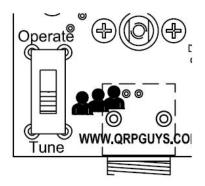
[ ] Install the hardware posts for the antenna wire and counterpoise, as shown in the figure below. The posts should extend1/2" below the surface of the board. Complete the installation by cutting off 1/8" from the open end of the two small vinyl caps and sliding them over the exposed threads of the posts.
