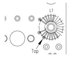
[ ] Secure L1 to the bottom side of the board using one of the 4-40 nylon screws, nylon washer, and nylon nut, as shown below. Tighten enough to secure and protect the toroid, but do not over tighten.
