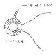
[ ] For L2, use the FT37-43 (black) core and 24" of the supplied magnet wire. You are winding a total of 25 turns, with a tap at 5 turns from the beginning of winding. Remember, every time the wire goes through the center of the core, it counts as one turn. Use the same twisted technique for the tap as L1. The total of 25 turns will completely fill the toroid.
