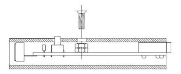
[ ] The two vinyl caps need to have a hole in them and installed on each end. For the microphone end, a 1/4" hole in the center will do. The 3.5mm jack end, 1/4" hole also, but you will see the jack is off center and the cap will need to match the offset jack. Use an xacto knife to cut the vinyl. It is soft and will cut easily.
