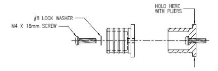
[] Press both PEX plugs into the 4" length of PEX pipe. Carefully measure and mark the PEX pipe as shown below, from each end of the assembly, and drill the six holes Ø3/32", through the PEX and aluminum to the inside only.
