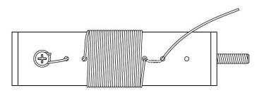
[ ] Again, remove 1/2" of the enamel insulation from the wire where the wire wraps around the screw and secure this end with the 6-32 screw and washer.
