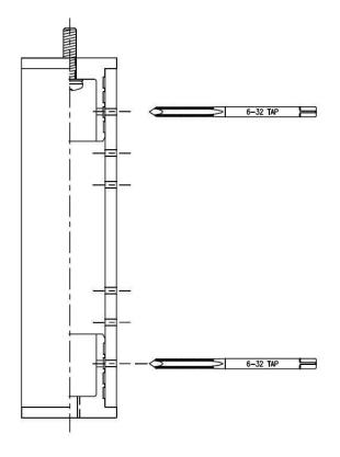
[] Mark the plug with the larger threaded hole and that end of the tube, so you don't mix the plugs after you drilled. Then remove both PEX plugs. Snake one end of the 22awg magnet wire into the hole shown, and back out the other hole. Re-install the PEX plug with the large threaded hole, and remove 1/2" of the enamel insulation from the wire and secure with the 6-32 screw and #6 washer with the wire *between* the washer and screw head as shown below.
