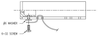
[] Wind a total of **51 turns**, close wound, and feed the far end of the magnet wire down thru the hole location shown to the inside, and back to the outside thru the next hole. You can now trim, leaving 3" of the 22awg magnet wire. Re-install the PEX plug, making sure the 6-32 hole aligns. *Double check your turn count. When counting coil turns, it is easy to make a mistake. I find it helpful to take a sharp, close-up picture, and print it. It's a lot easier to count.*
