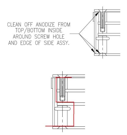
Route a single strand of bare wire (.005-.008") from a short piece of #24 or 26awg stranded wire as shown tying the three cleaned surfaces to the ground around the pcb hole. Clip the strand flush where is exits the case.
