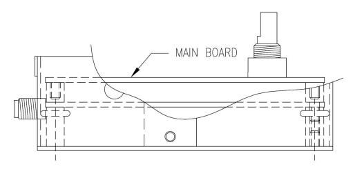
[ ] Loosely install the two M3 x 5mm thin pan head screws into the side assembly. The o-rings will act as centering devices for the side assembly. Squeeze the side assembly against the o-rings and tighten the two pan head screws.
