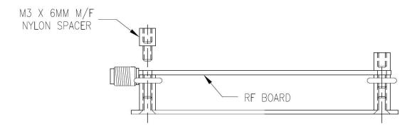
[ ] Carefully spring open the side assembly enough to place around RF board allowing the SMA and other I/O connectors to protrude through the side assembly. Do not install the screws to the side assembly yet.
