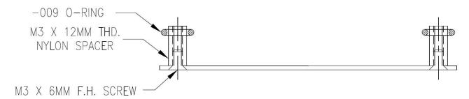
[ ] Place the RF board on the four M3 x 12mm nylon spacers and secure with the M3 x 6mm M/F nylon spacers.
