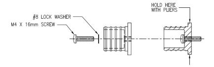
[ ] Press both PEX plugs into the 4" length of PEX pipe. Carefully measure and mark the PEX pipe as shown below, from each end of the assembly, and drill the six holes Ø3/32", through the PEX and aluminum to the inside only.
