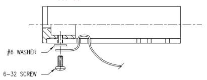
[ ] Wind a total of **51 turns**, close wound, and feed the far end of the magnet wire down thru the hole location shown to the inside, and back to the outside thru the next hole. You can now trim, leaving 3" of the 22awg magnet wire. Re-install the PEX plug, making sure the 6-32 hole aligns. Double check your turn count. When counting coil turns, it is easy to make a mistake. I find it helpful to take a sharp, close-up picture, and print it. It's a lot easier to count.
